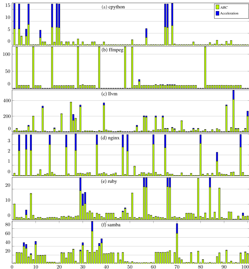
Fig. 4. Acceleration of ABC. x -axis denotes incremental builds while y -axis denotes time (in seconds).
